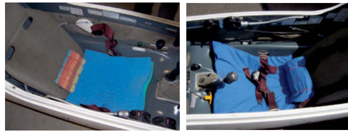
Figure 5. The left picture shows the two layers of Confor C47 and C45 that were used to make up the seat cushion. The right picture shows the covered cushion in position. A lumbar support made out of the same materials can also be seen. Note that the manufacturer's supplied cushions were removed
