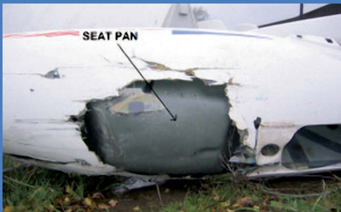
Figure 1. Underside of a glider cockpit following a crash, revealing the close proximity of the seat pan to the outer skin of the glider and therefore the limited seat structure available to help absorb energy
