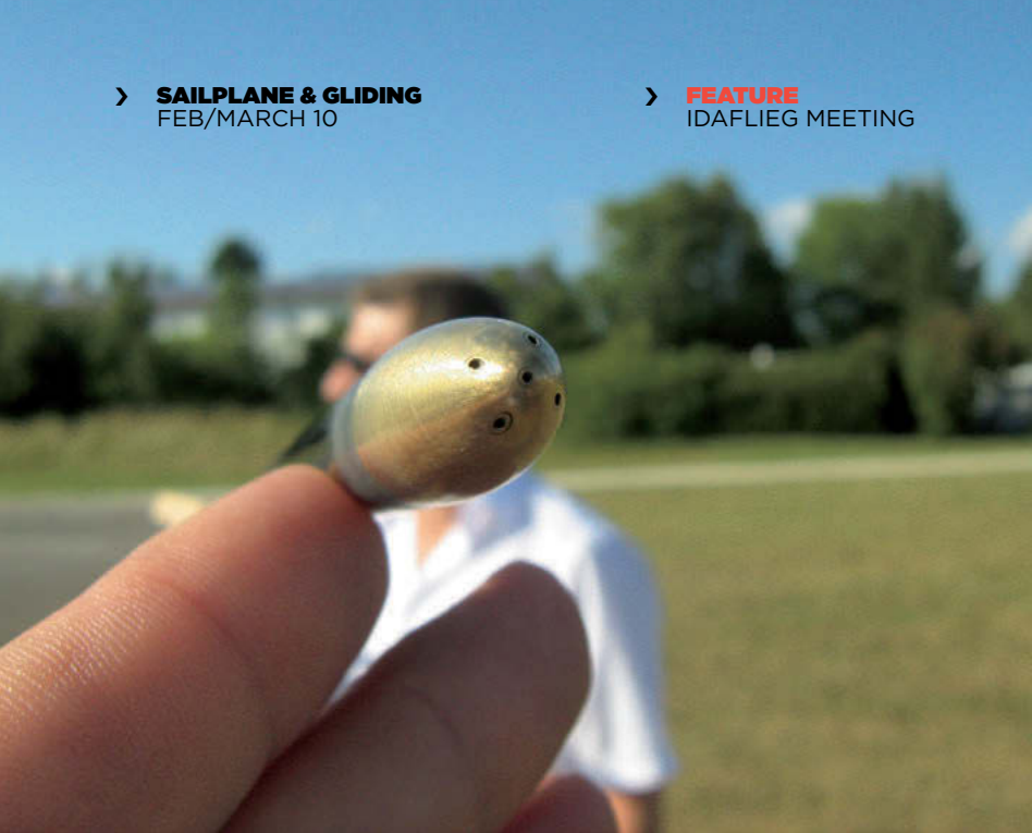
An infrared camera (above right) takes a 'digital film' of the wing surface of the Dresden Akaflieg Twin Astir. The data of the approaching airflow is measured by a five-hole probe (above left) mounted at a gallows at the wingtip, which enables measurement of angles of sideslip and attack. (Below) Falk Paetzold of the IFF tests a special helmet to detect the pilot's view and eye movements in flight (All photos by Jochen Ewald)
