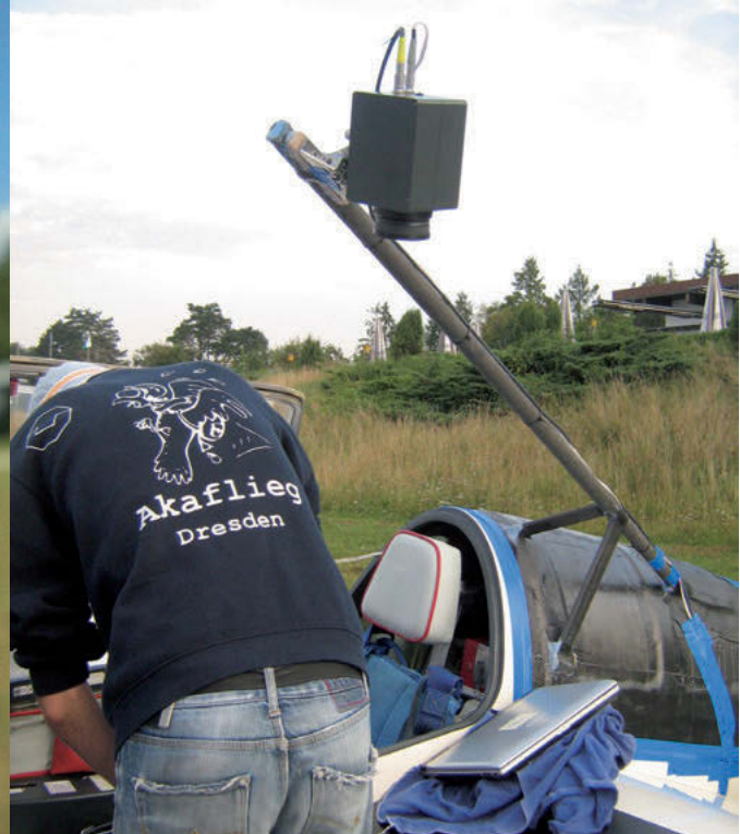
An infrared camera (above right) takes a 'digital film' of the wing surface of the Dresden Akaflieg Twin Astir. The data of the approaching airflow is measured by a five-hole probe (above left) mounted at a gallows at the wingtip, which enables measurement of angles of sideslip and attack. (Below) Falk Paetzold of the IFF tests a special helmet to detect the pilot's view and eye movements in flight (All photos by Jochen Ewald)
