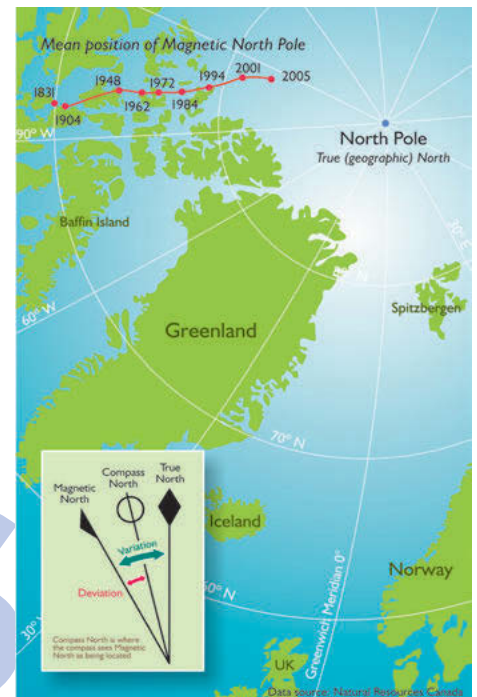
(Above) Figure 4: Variation UK (Below) Figure 5: Movement of Magnetic North
