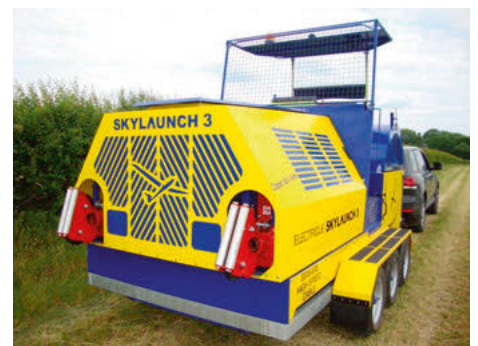
Skylaunch's fully electric winch has been in operation in France since 2011
