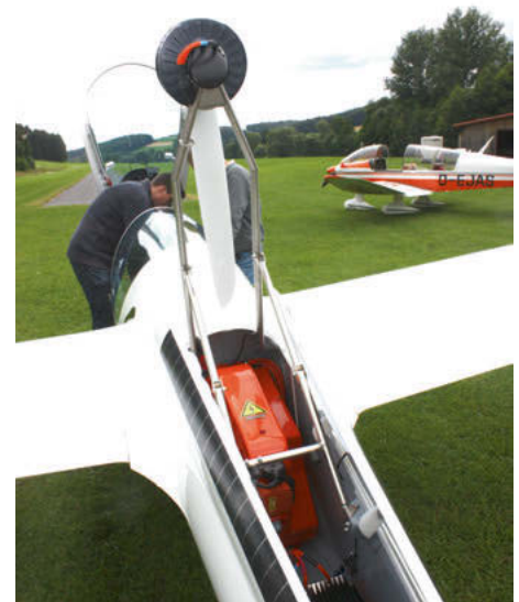
Location of battery pack in the front of the engine bay (Bernard Eckey)
