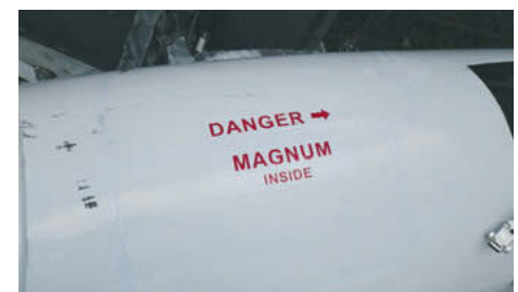
Warning sign affixed to BPRS compartment access panel
