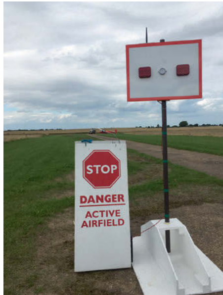
Traffic lights connect to winch and launch point
