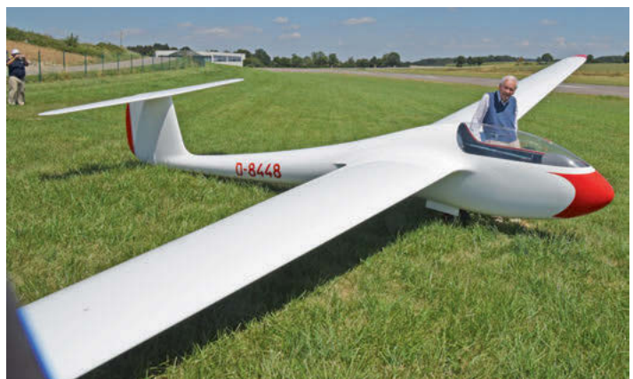
Below right: The Phönix T is the first small serial production sailplane built by Richard Eppler, Hermann Nägele and Rudolf Lindner with glass-fibre composites. In this photo, Prof Dr Richard Eppler stands next to the Phönix T, originally owned by Hermann Nägele
