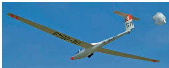
The Kestrel was Glasflügel's first aircraft in the Open Class. As part of the serial production, the ship was equipped with a drag parachute for steep short landings.
