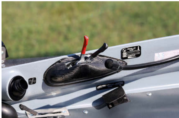
Above: gas lever and propeller stop in the same console Below: fail safe fuel indicator
