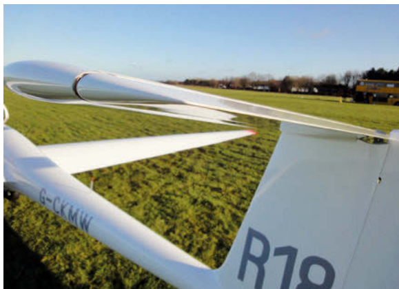
Fin ballast can correct the C of G (see glider manual) and alleviate unwanted up-elevator drag. It also improves manoeuvrability in turns (Kevin Atkinson)
