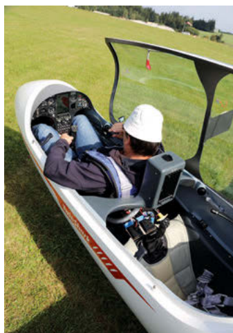
EB28 cockpit modified for tall and generous build pilots
