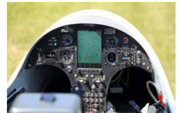
Gear up/down indicator to the left and ILEC engine control on the right side
