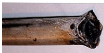
View of the inboard end of the centre aileron push rod from the left wing showing localised heating, part of the fork end fitting and undistorted tube section
