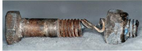
Lower bolt failure
