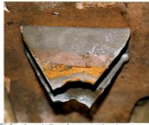
Right aileron bellcrank mounting bracket showing melted end and heat effects
