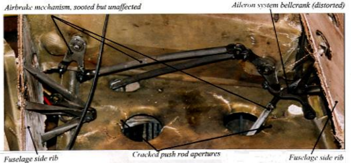
Controls in fuselage centre section, illustrating extent of sooting
