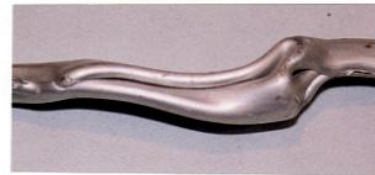
Details of centre push rod from right wing Rod is normally a tube of 16mm diameter, 1mm wall thickness
