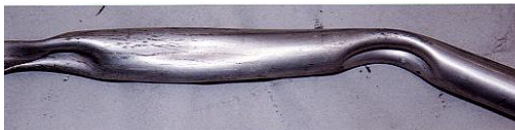
Above and below, outboard end of centre push rod illustrating crushing and arcing damage at outer end only
