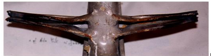
Crossbeam showing symmetrical nature of deformation/damage from Joule heating
