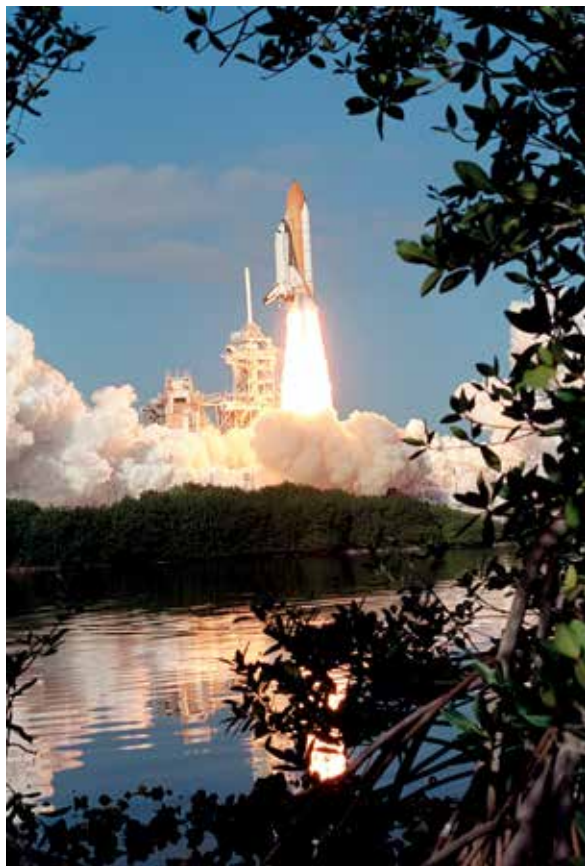
During the lift-off of Space Shuttle Columbia on 16 January 2003 a piece of foam insulation broke off, hitting a wing. The problem was spotted, but not acted on possibly because failure of the foam insulation had become the norm (photo courtesy of NASA)
