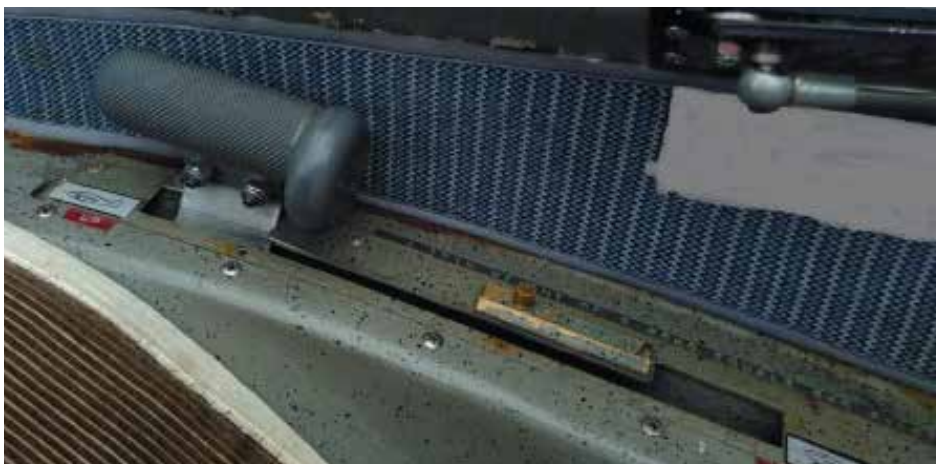
In the LS8 pushing the undercarriage lever forward puts the wheel up!
