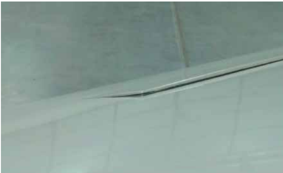
Astir airbrakes closed but not locked. The ground crew should check this before attaching the cable for launch.
