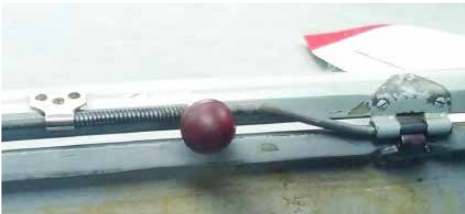
Astir canopy locking pin has missed the hole
