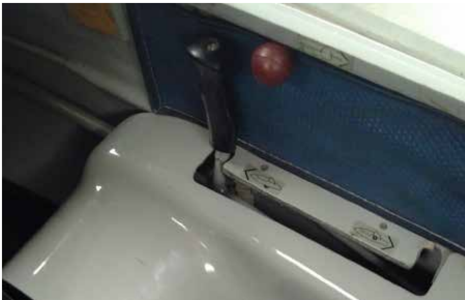
In the Astir pushing the undercarriage lever forward puts the wheel down
