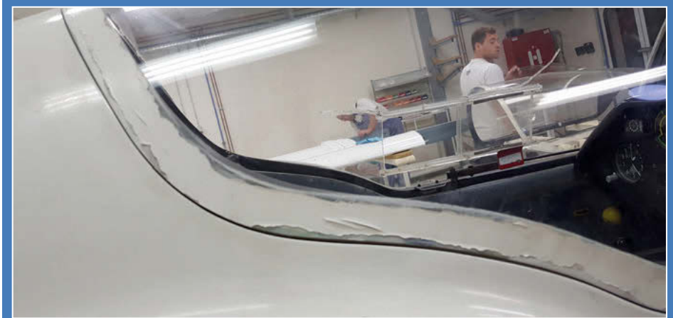
Top: Showing poor canopy fit and gaps Left: Serious gaps around front canopy Right: Cracks and scratches in the glass skin (All photographs courtesy of GliderService Novak)
