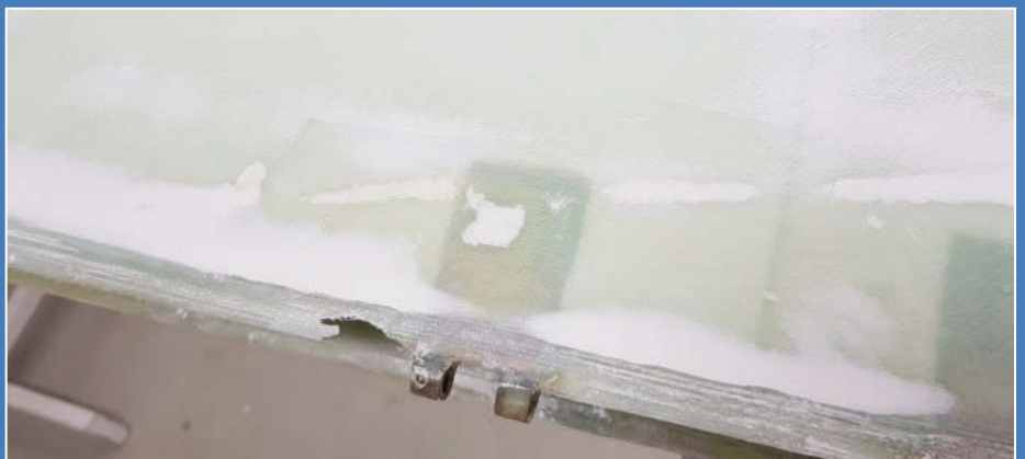
Damage on the TE of the tailplane
