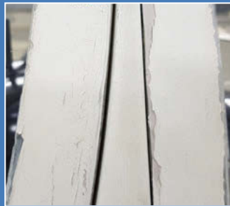
Top: Showing poor canopy fit and gaps Left: Serious gaps around front canopy Right: Cracks and scratches in the glass skin (All photographs courtesy of GliderService Novak)
