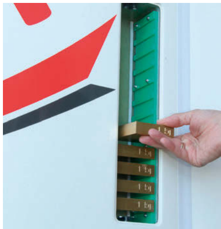
(Below) Spin ballast – cube-shaped brass weights are placed into a box integrated into the fin
