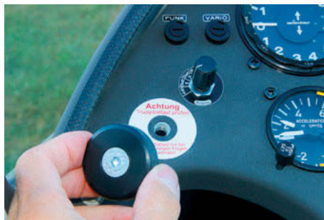
(Above) Fixing bolt for spin ballast
