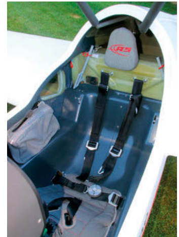
(Above) Back seat: a new headrest and new attachment for fastening straps, for improved crash safety
