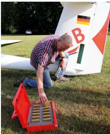
Schleicher's Ulrich Kremer with spin ballast – a fin ballast box is available as an optional extra
