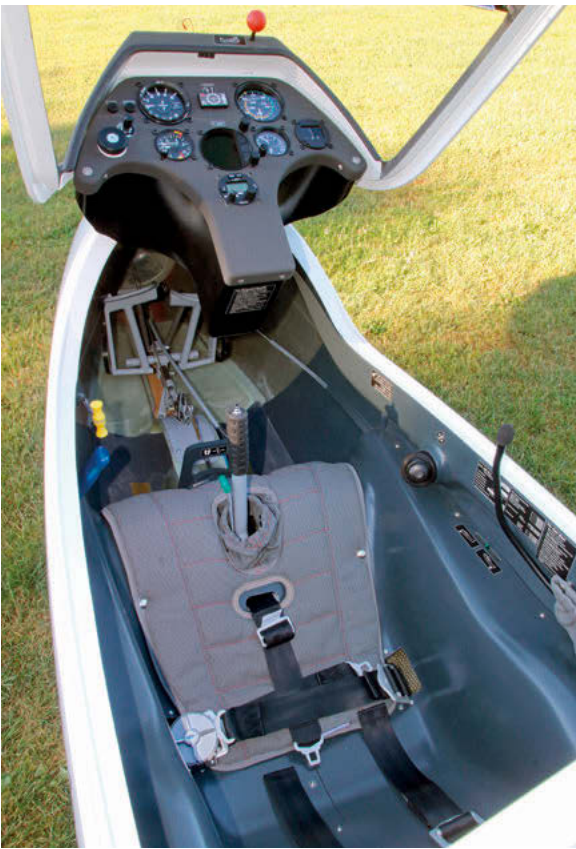
(Left and above) Front seat: the instrument panel has been slightly modified, allowing space for larger pilots and better seating comfort. The seat cushions are new and filled with Dynafoam
