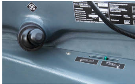
(Below) New ventilation outlets are easier to adjust and aim. The noise level is also reduced
