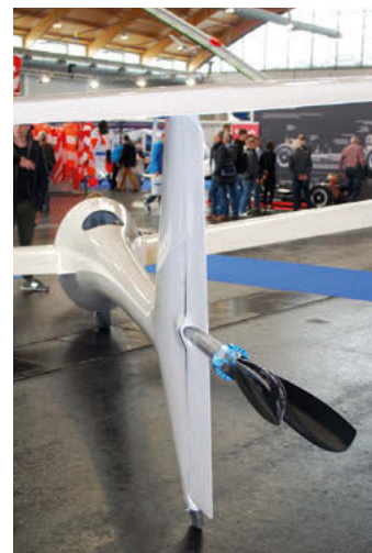
The foldable propeller of the Birdy, a motor glider in the 120kg class
