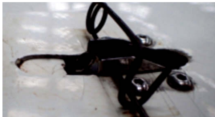
Locking lever when tailplane attached (above left) and when locked with safety pin inserted (above right)
