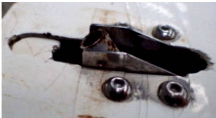
Locking lever when tailplane attached (above left) and when locked with safety pin inserted (above right)
