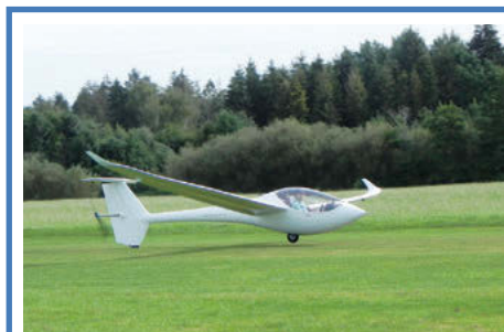
The Birdy high-performance motorglider in the 120kg Class; wing profile by Loek Boermann
