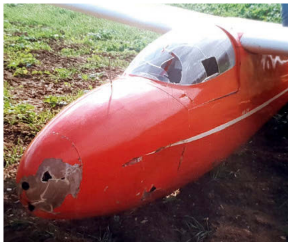
Crash damage after Bymbo hit a tree in 1999 resulted in a major rebuild
