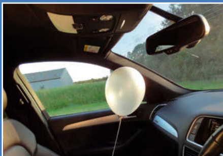
Fig 1: As the car accelerates, the helium balloon is driven forward by the denser air
