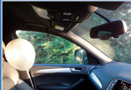
Fig 2: As the car slows, the helium balloon is driven backwards by the denser air
