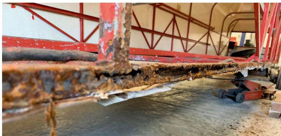
Above and below left: corrosion on the steel frame in JAL's trailer and, below right, the newly-replaced box section (photographs by Harriet Gamble)
