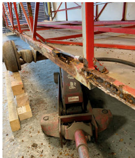
Above and below left: corrosion on the steel frame in JAL's trailer and, below right, the newly-replaced box section (photographs by Harriet Gamble)
