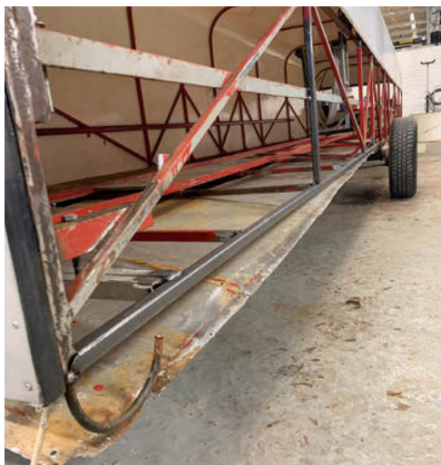
Above and below left: corrosion on the steel frame in JAL's trailer and, below right, the newly-replaced box section (photographs by Harriet Gamble)
