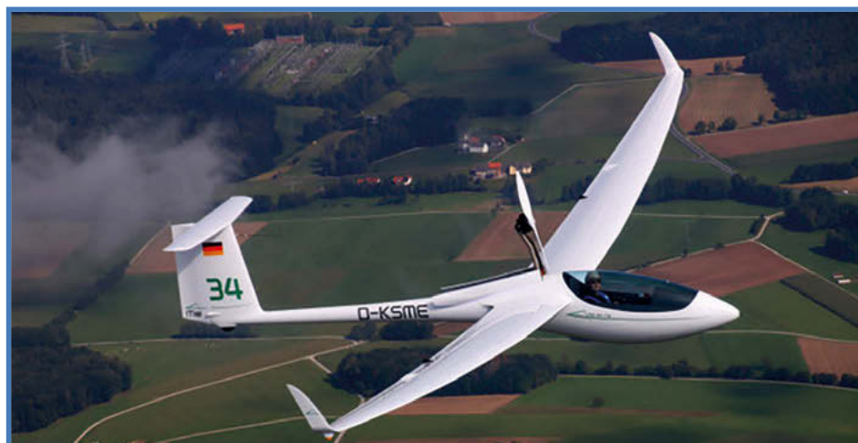
■ Schleicher's AS 34 Me pictured during its maiden flight in September. Managing director Uli Kremer said: "We have added an electrically-powered self-launching Standard Class aircraft to our product range, which is primarily designed for pilots who prefer a simple to fly, simple to maintain and simple to operate aircraft on the ground and in the air. As long as they can find a power outlet at the end of the day they can expect a fully operational aircraft when next they arrive at the airfield."
